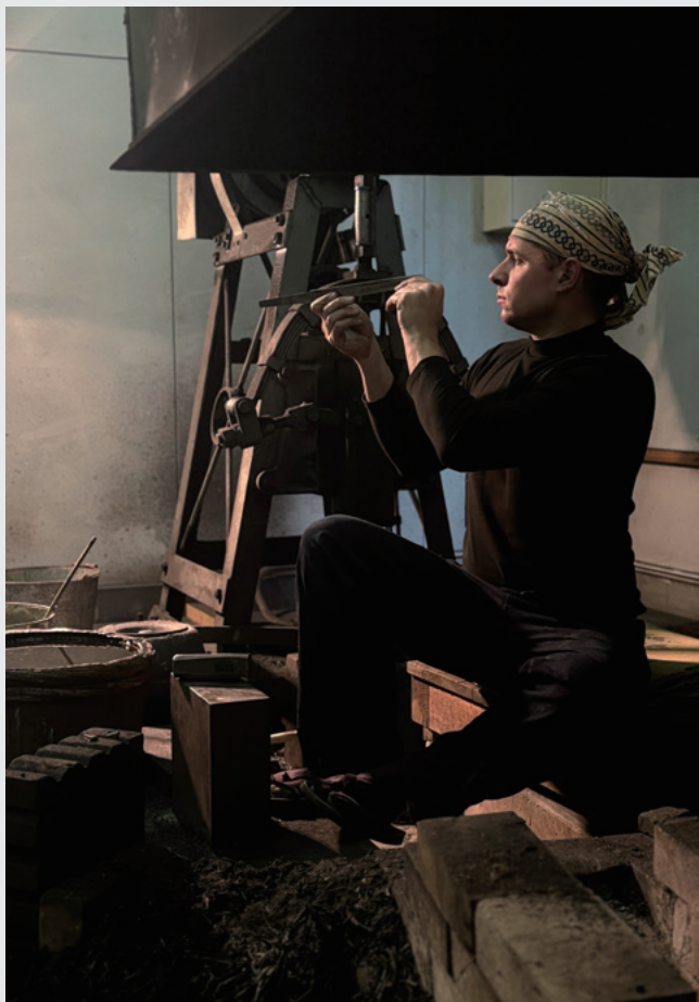
Adjusting and finishing the curvature of the tanto (dagger).
