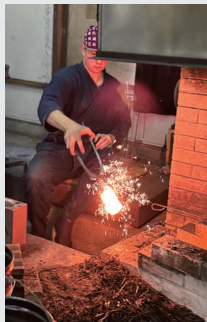
The raw material for a Japanese sword, tamahagane , 3 is heated to over 1,200°C and hammered to remove impurities.
